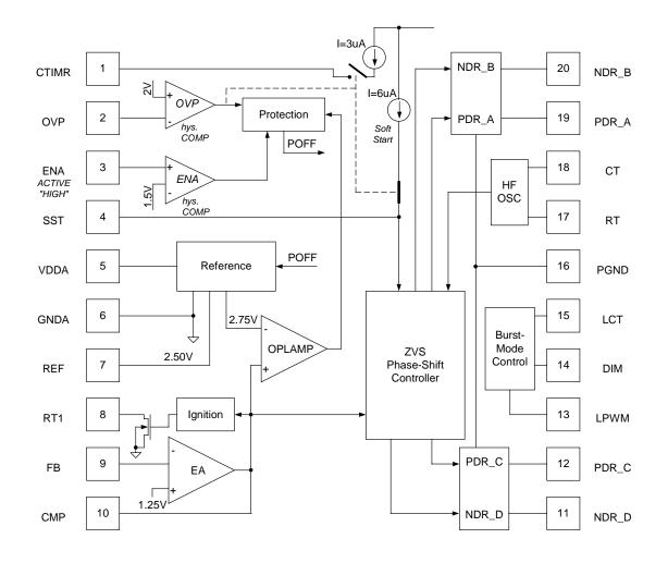
Figure 2. Functional Block Diagram
