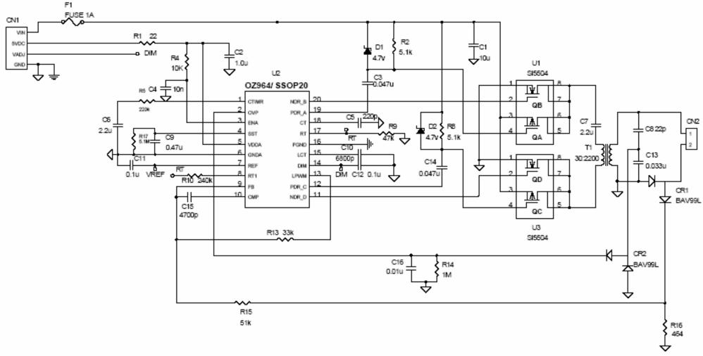
VIN: 8.0V - 22V VADJ: 2.1V Max. Brightness; 0.6V Min. Brightness Striking frequency: 75.1KHz Operating frequency: 63KHz 5VDC: 4.75V - 5.25V
